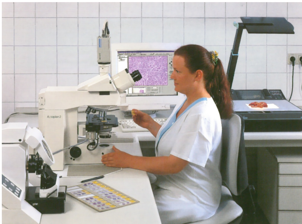
The Visualizer is used to record the removed tissue and transfer the image via video conferencing directly onto the computer screen of the remote expert.
