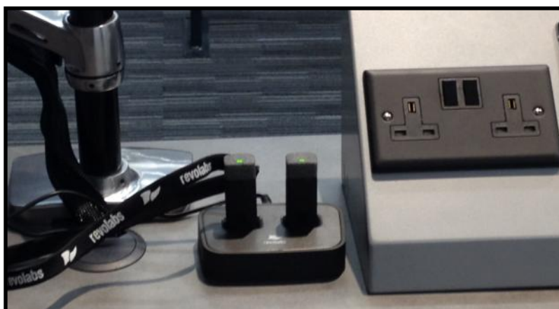
Revolabs HD-based Wireless Microphones 'Out of the charger is on, and back in is off'.
