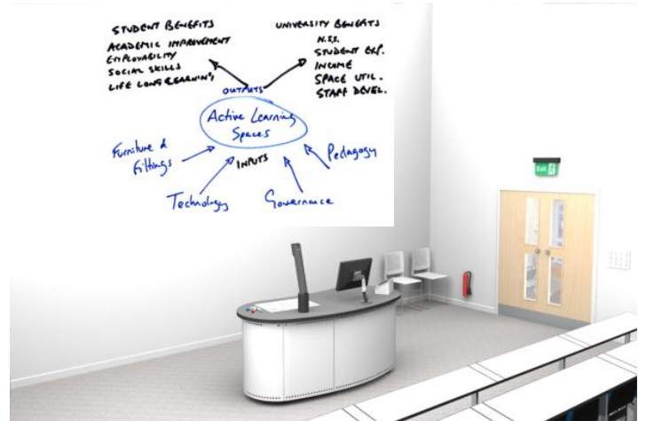
Sketch of a Lecture Theatre at Warwick Business School where a WolfVision ceiling-mounted Visualiser captures and displays the content from a dry-wipe surface in a TOP-TEC Lectern.
